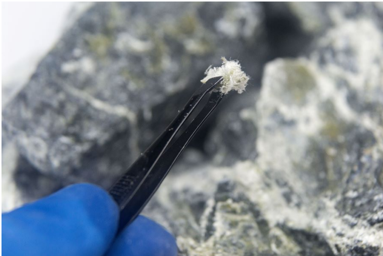
When disturbed, the tiny asbestos fibers are easily inhaled and become lodged in the lungs.
